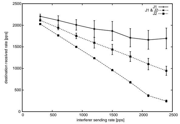
**Figure 10: The amount of interference is linear with respect to interferer rate. Separate interferers acting simultaneously also create interference that is linear with their combined rate.**
