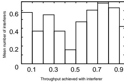
**Figure 6: Histogram of the number of interferers for each interval of achieved throughput. Interferers allowing more than 95% of the throughput are omitted. The sum of the first two bins shows that there is on average one interferer reducing the capacity to 20% or less.**
