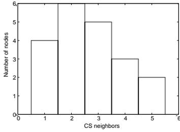
Figure 3: Histogram of carrier sense (CS) degree of nodes - on average, 2.6 nodes are within CS range in a mesh of 20 nodes.
