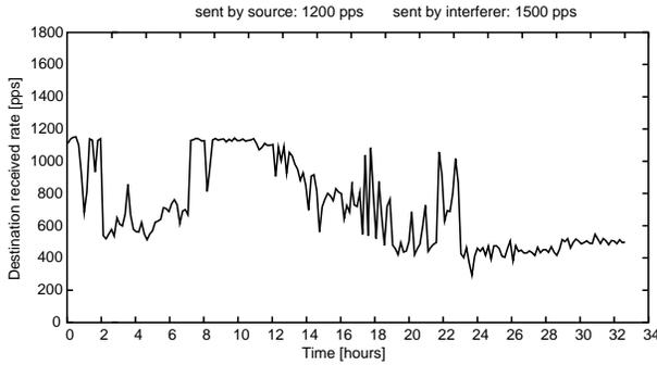
**Figure 7: Time line: due to external factors, interference measurements taken at different times cannot be compared. We use a round robin scheme to alternate between measurements and identify stable periods, which allow for meaningful comparisons.**
