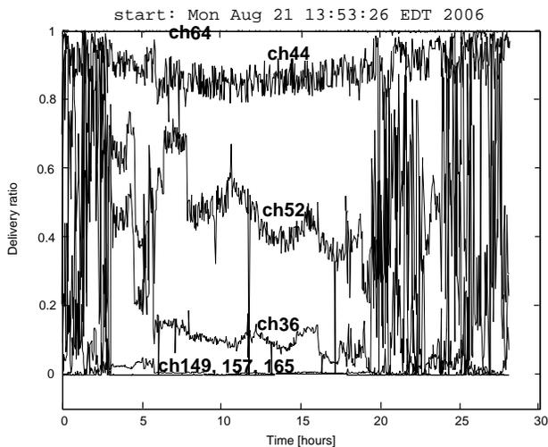
**Figure 18: Delivery ratio differs widely across channels. Channel allocation algorithms may not assume that channels are interchangeable in terms of performance.**
