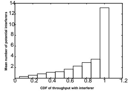
Figure 5: Cumulative distribution of the number of possible interferers and the amount of damage they produce. Nodes outside interference range are not included. On average, there are 2 interferers which reduce the capacity of the link to 60% or less.
