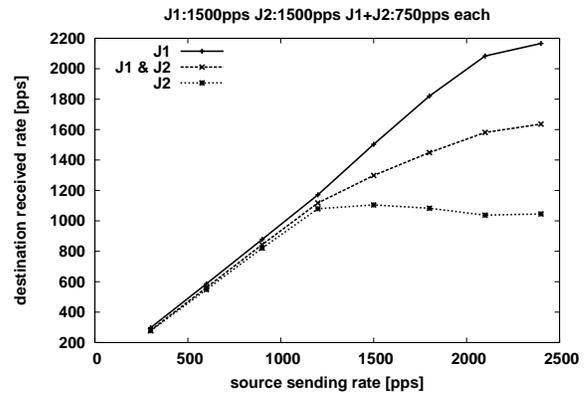
**Figure 11: Even with anomalies in power of emitted packets, effect of interferer is linear with respect to sending rate for single interferers, and for combinations of two.**
