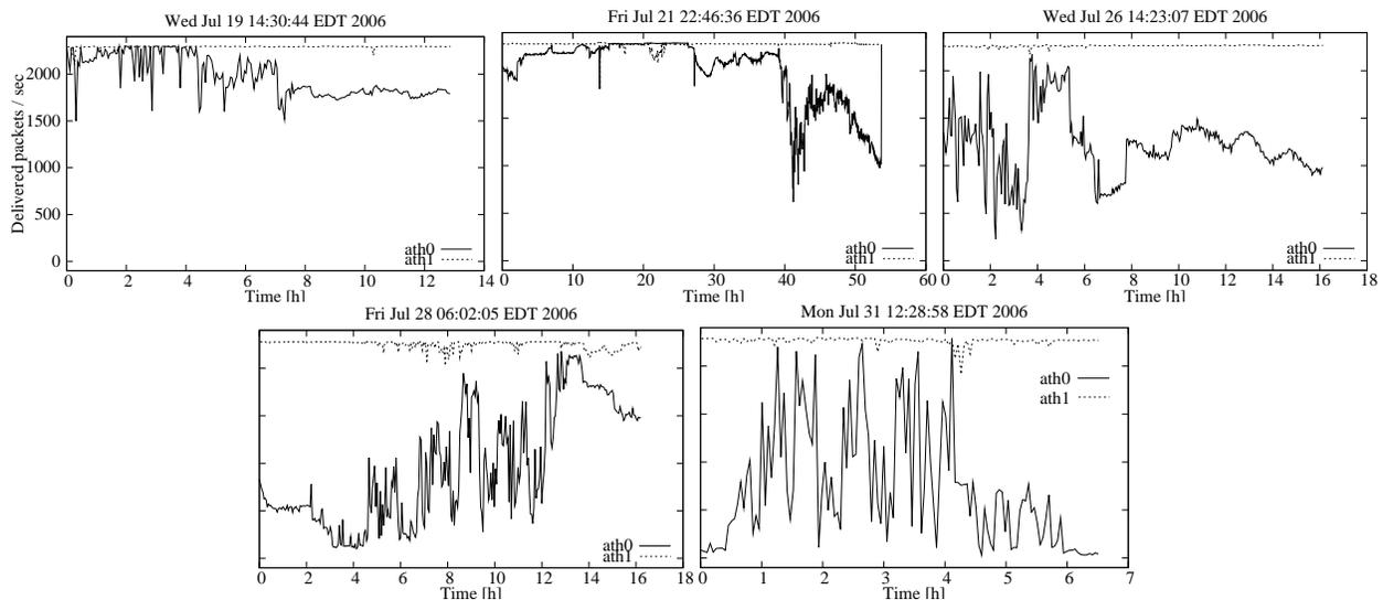
**Figure 17: Delivery ratio sampled for a total of 110 hours spread over a period of two weeks. Delivery ratio differs widely across interfaces. Channel allocation algorithms may not assume equivalence of link performance based on sampling of links from a single interface.**
