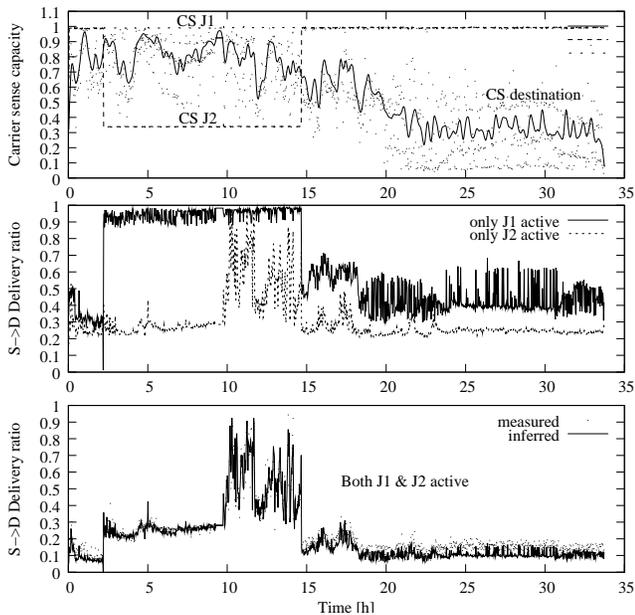
**Figure 12: Top: History of access to the medium for the interferers and the destination. Middle: delivery ratios sampled independently for each interferer. Bottom: When both interferers are active, measured delivery ratio confirms the independence of the two interferers .**
