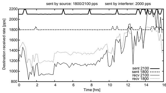
**Figure 9: Anomaly: packets sent at higher rate use a lower signal strength, yielding in a lower delivery ratio. This behavior is persistent for many hours.**
