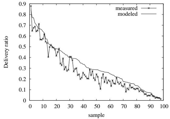
**Figure 13: A source and two interferers send data at random rates - we sort the experiments based on delivery ratio achieved. Using equation (2), we predict the delivery ratio based on separate measurements for each interferer. The correlation is quite high (0.97) but the model overvalues the delivery ratio by about 4.5%.**
