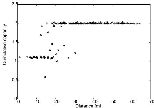
Figure 15: Carrier sense depends strongly on distance.
