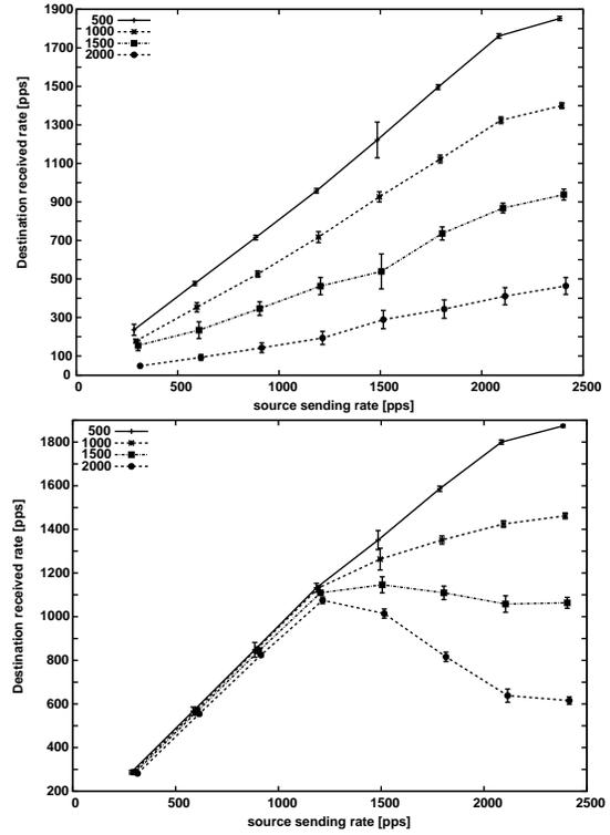
**Figure 8: Delivery rate with one interferer. Top: in most cases, the achieved throughput in packets per second is linear with the sending rate for the entire range of sending rates. Bottom: low rate flows from the source are not affected by the interferer, but for higher rates, the behavior is still linear.**
